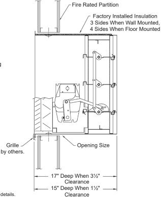
Combination Fire/Smoke Damper ▲ 1½ Hr. Rated ▲ Single Thickness Blades ▲ Leakage Class II ▲ 250°F or 350°F Rated ▲ Front Access Grille ▲ Galvanized Steel
